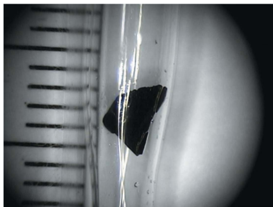
Figure 1 The crystal of equine cyanomethemoglobin used for the neutron diffraction data collection. The crystal measured about 3.5 \times 2.5 \times 1.2 mm in size ( \sim 10 mm 3 ) and was mounted in an hourglass-shaped quartz capillary.
